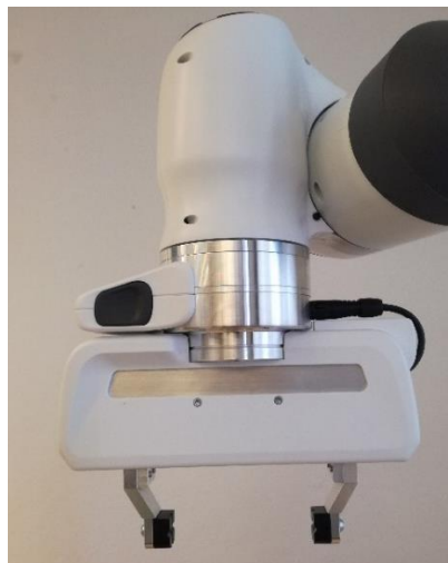
Figure 3 - Robot gripper with standard fingers from Franka Emika
